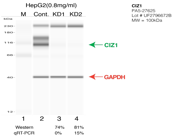
Figure 3: Western Blot Analysis of depletion level of the target RNA binding protein in control and knockdown cells. Lane 1: Molecular weight marker. Lane 2: 30 \mu g of protein from HepG2 transduced with a control, non-target gRNA (ENCODE Biosample ENCSR306EWE and ENCBS217OPS). Lane 3: 30 \mu g of protein from HepG2 transduced with a gRNA targeting CIZ1 (ENCODE Biosample ENCSR749QMU). Lane 4: 30 \mu g of protein from HepG2 transduced with a gRNA targeting CIZ1 (ENCODE Biosample ENCBS100NPF). Samples were separated by SDS-PAGE, transferred to a membrane and blotted using antibodies against CIZ1 (ENCODE Antibody ENCAB411FAE) and GAPDH as controls.
